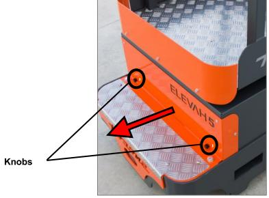
When the step is completed, set the protective casing of the base back in place and tighten the knobs again.
