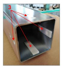
3. Remove all the pads (4) present (4 on each side) in the upper part of the second extension, fully extract it from the column and remove the four pads (5) in its lower part;
