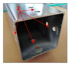
4. Insert four new pads, on each side, in the holes (3) made externally, at the top of the second extension;
