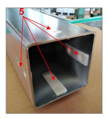
4. Remove all the pads (6) present (4 on each side) in the upper part of the first extension (directly connected to the machine base);
