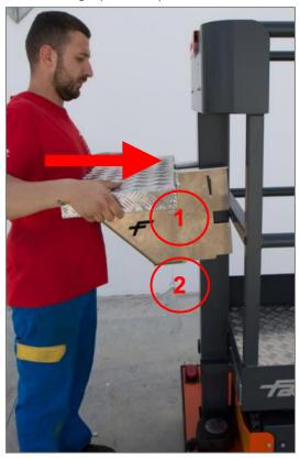
Insert the locking bracket (secured to the surface) in the specific hole, until it engages in the grooves.
