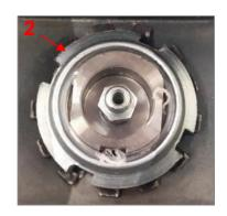
2. Lift the cage unit using a winch or other lifting equipment, completely extracting the third extension (part of the cage unit) from the column and remove the four pads (3) on it;
