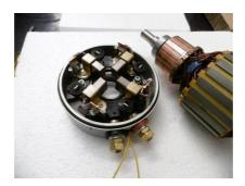
7. Measure the groove of the manifold and the length of the brushes.
