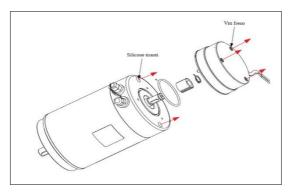
3. Mark the contact surface of the tube with the shield and the flanges to the restore proper alignment;
