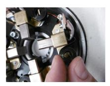
b. Unscrew the fixing screw (1) and extract the brushes (2);
