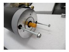
5. Extract the rear shield with the brush holder (using a rubber mallet if necessary) paying attention not to ruin the o-rings between the tube and the shield/flanges.
