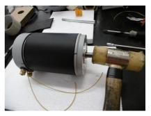
6. Extract the brush holder and clean the manifold and the adjacent area with compressed air
