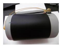
4. Unscrew the motor tie rods using a 10 [mm] socket wrench
