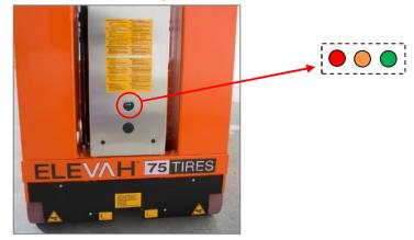
While recharging the battery, the **RED LED** indicates the beginning of the charging cycle. Charging stops automatically with no need for operator action, and is indicated by the **GREEN LED** on.
