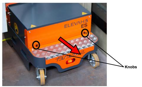
When the step is completed, set the protective casing of the base back in place and tighten the knobs again.
