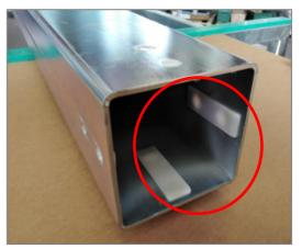
Insert eight new pads into the holes (2) made externally, on each side, at the end of the first extension;
