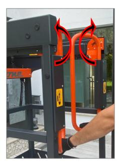
Access the cage by lifting the mobile doors slightly by pushing and rotating them inwards. Once the operator enters, he/she must close the gate, checking that the gate itself is locked properly, otherwise the machine will not enable any command.
