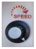
When the machine is in transport position (cage fully lowered), it is possible to regulate the transmission speed from the regulator. By turning the regulator anti-clockwise it is possible to lower the translation speed. On the other hand, by turning the regulator clockwise it is possible to increase the translation speed.
