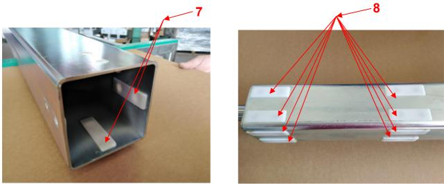
4. Remove the old layer of grease and clean the surfaces.
